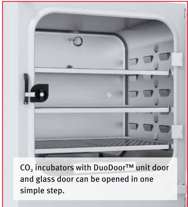
CO<sub>2</sub> incubators with DuoDoor™ unit door and glass door can be opened in one simple step.
